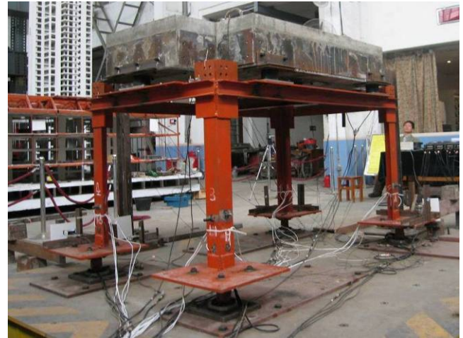
Fig.4 Photo of the frame modal in the FIED structural system setting on the shaking table
