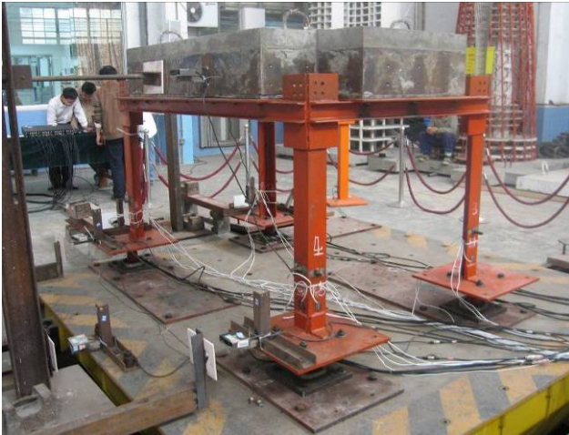
Fig.3 Photo of the frame modal in traditional system setting on the shaking table
