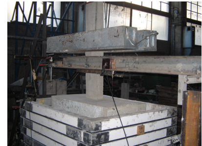
Fig. 6c. Model pier and 2 nd shear stack tested at the Laboratory.
