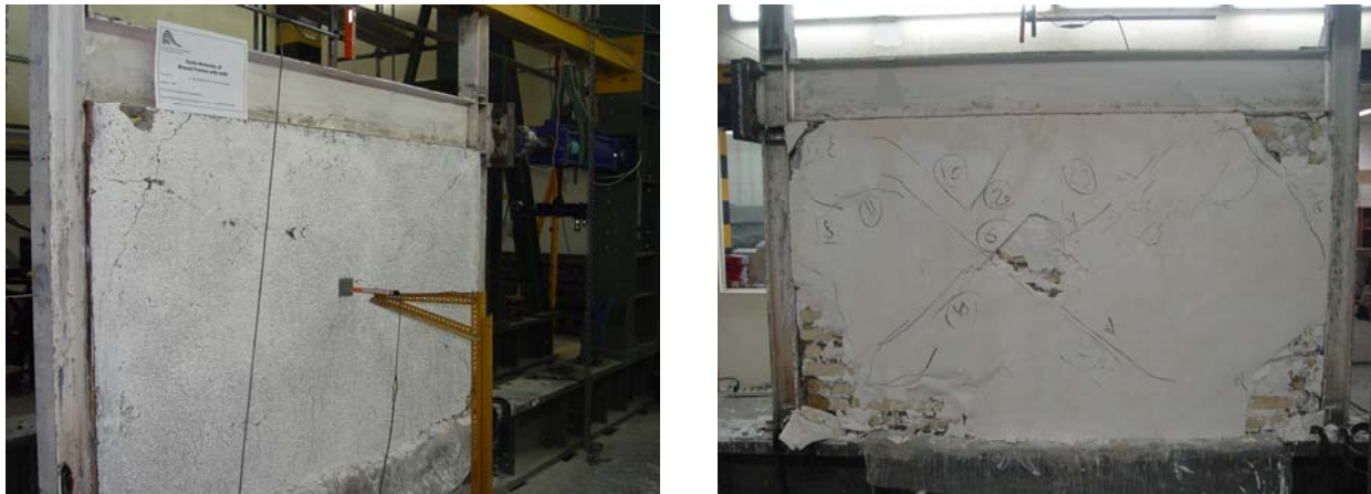
Figure 3 Crack developments on each of the two sides
