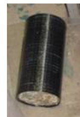
(a) Specimen with primer layer (b) Specimen with putty layer (c) CFRP wrapped specimen
