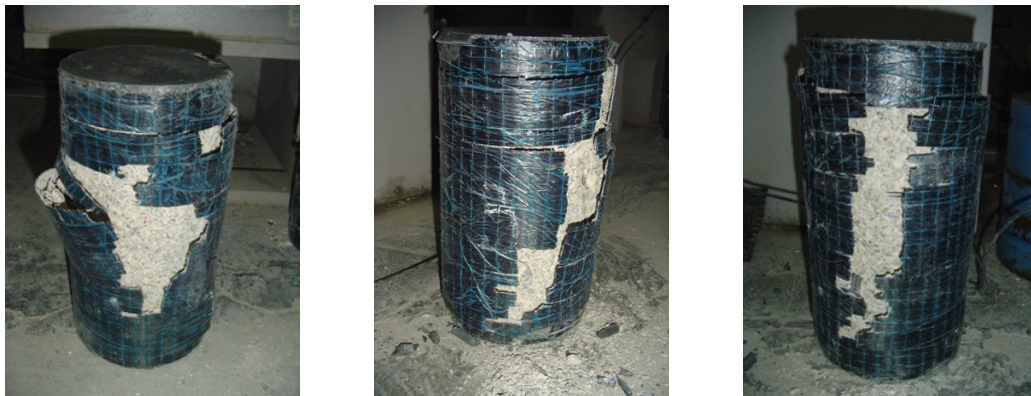
Figure 5: Typical views of low-strength concrete specimens after compressive strength tests
