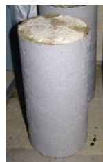
(a) Specimen with primer layer (b) Specimen with putty layer (c) CFRP wrapped specimen
