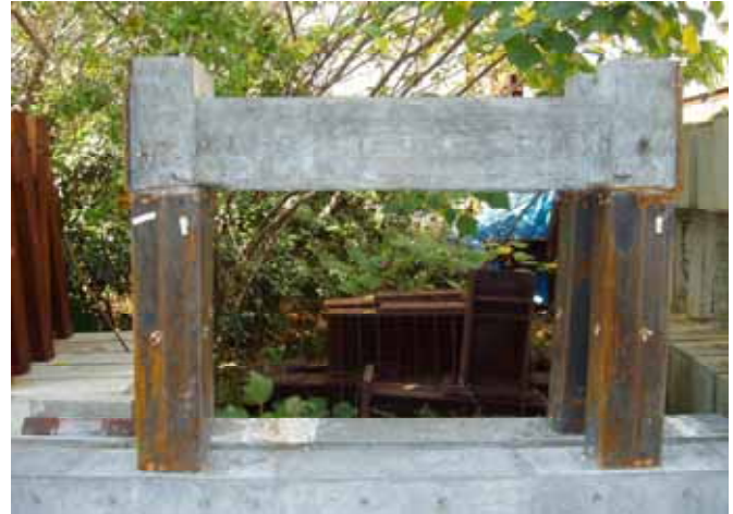
Photo 2 Frame with Ultra High-Strength Rebars
