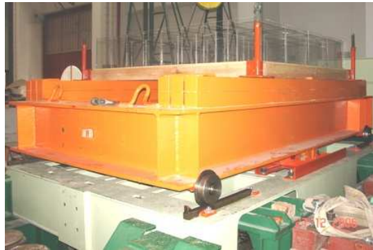
Figure 2. Testing set-up of the transmission system with 32 TLDs included [Falcão Silva et. al, 2007]
