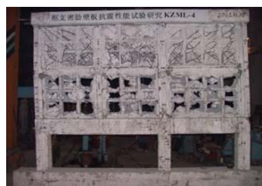
Figure 9 Failure phenomena of KZML-4
