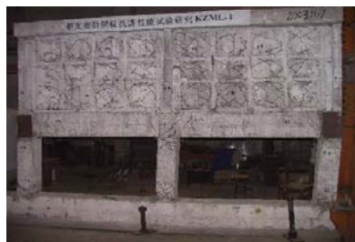
Figure 6 Failure phenomena of KZML-1
