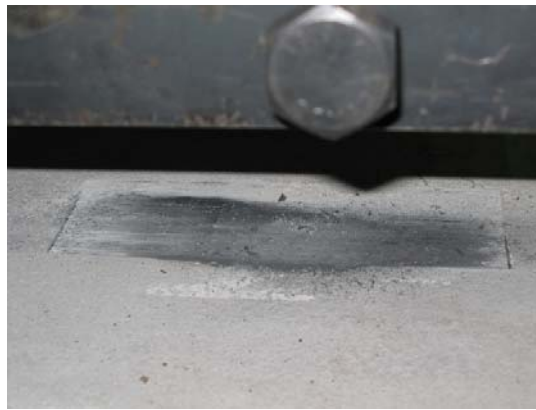
Fig 2 Scraped mortar plane surface
