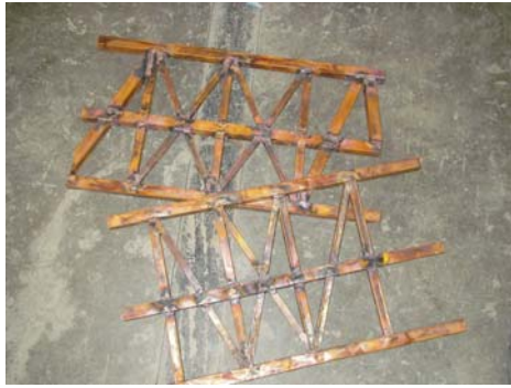
Photo 2 consolidation of single piece of truss
