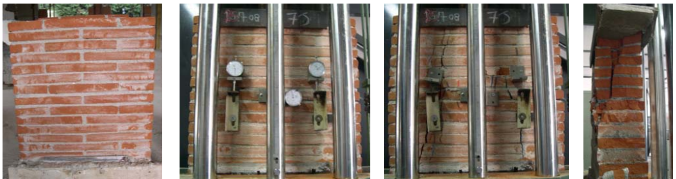
Figure 12 Brick panel: sample, instrumentation, external and internal crack pattern
