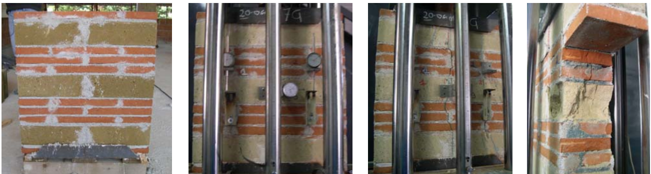
Figure 10 Multiple Tuff-Brick listed panel: sample, instrumentation, external and internal crack pattern
