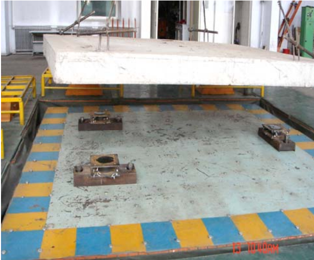
Figure 1 SMA wire-laminated rubber combined bearing
