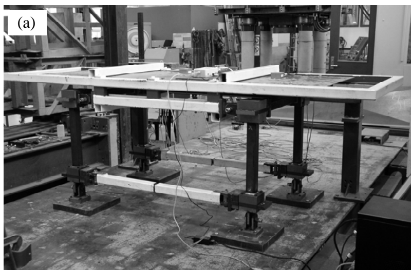
Figure 1. Photo of the mounted shake-table model structure in the torsionally restrained configuration.
