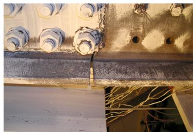
(a) MRF-1B, bottom flange fracture
