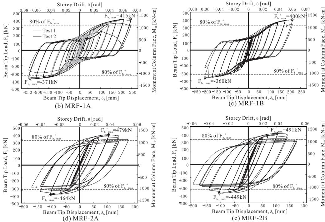
Figure 3.4 Hysteretic response of MRF specimens
