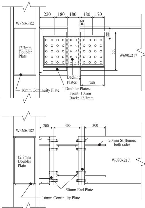
Figure 2.2 MRF beam-to-column joint details
