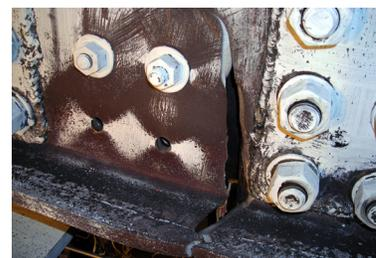
(b) MRF-1A, tear in web and bottom flange
