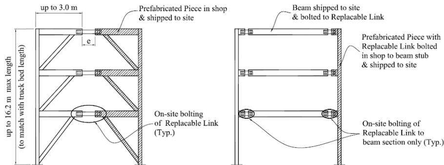
Figure 1.1 Replaceable link concept for: (a) EBFs, (b) MRFs
