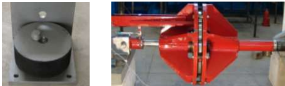
Figure 2 Elastomeric bearing (left) and magneto-inductive energy dissipation device (right) used in the tests.
