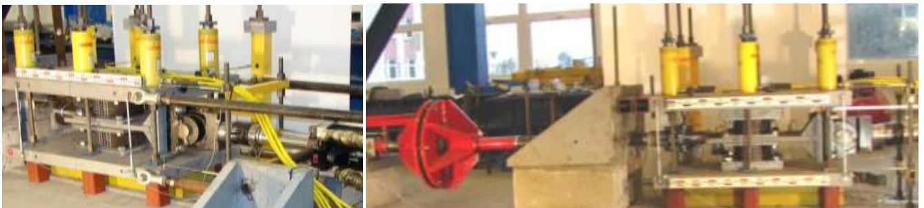
Figure 4 Experimental set-up for testing: elastomeric bearings (left), elastomeric bearings combined with magneto-inductive device (right)
