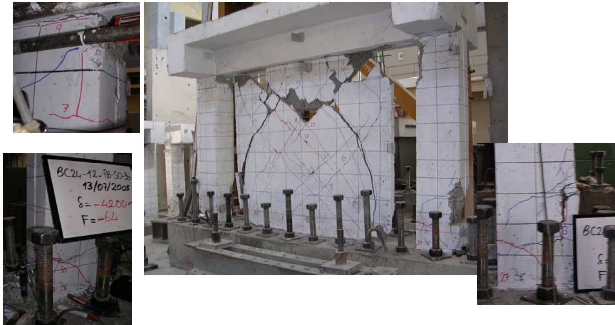
Figure 8 S2 after failure
