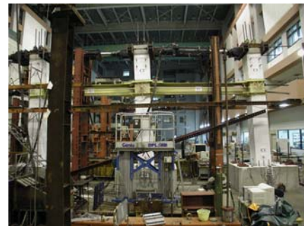
Figure 9 PT frame deformation (4% drift)
