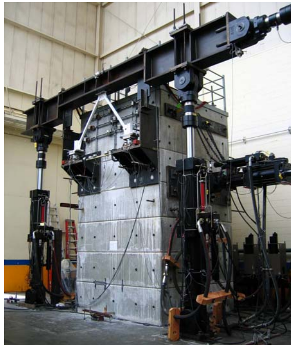
Figure 2: Test setup for the suspended zipper braced frame hybrid simulation at the nees@berkeley laboratory.
