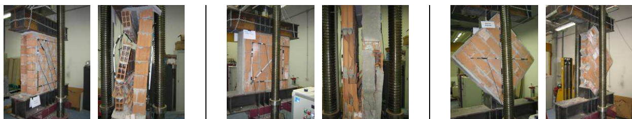
Figure 3.3 Double panels with mortar type 1: compression test results in strong, weak and diagonal directions
