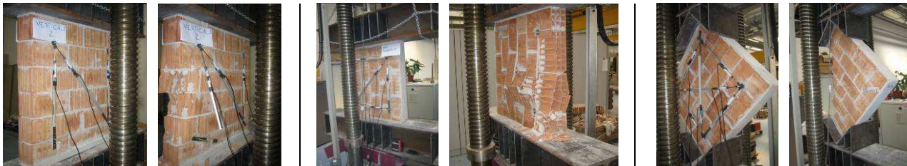
Figure 3.4 Half-full panels with mortar type 2: compression test results in strong, weak and diagonal directions
