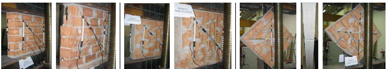
Figure 3.2 Half-full panels with mortar type 1: compression test results in strong, weak and diagonal directions
