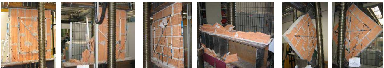
Figure 3.2 Hollow panels with mortar type 1: compression test results in strong, weak and diagonal directions
