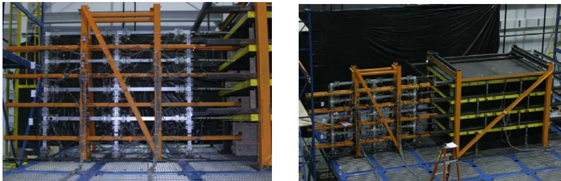
(a) test frame (b) 4-story test frame and mass simulator Figure 3. 4 story test frame on shaking table at the University at Buffalo NY after installation
