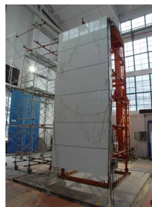
Figure 6 Shake table tests of curtain walls
