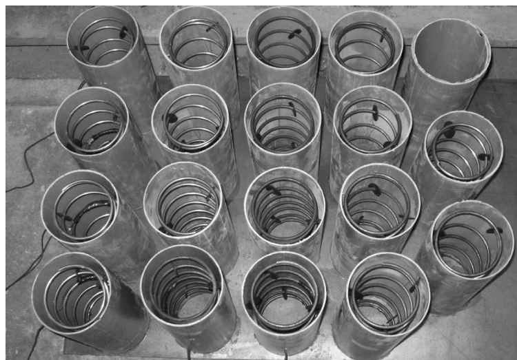
Figure 1 Molds of spirally reinforced specimens
