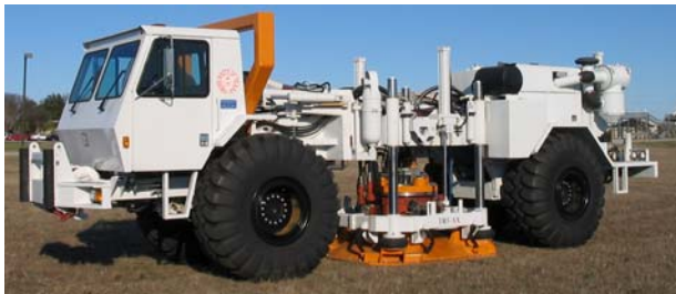
a. High-force, three-axis shaker called T-Rex
