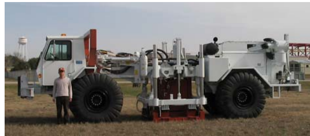
b. Low-frequency, two-axis shaker called Liquidator
