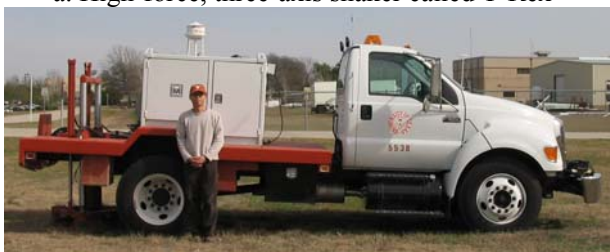
c. Urban, three-axis shaker called Thumper
