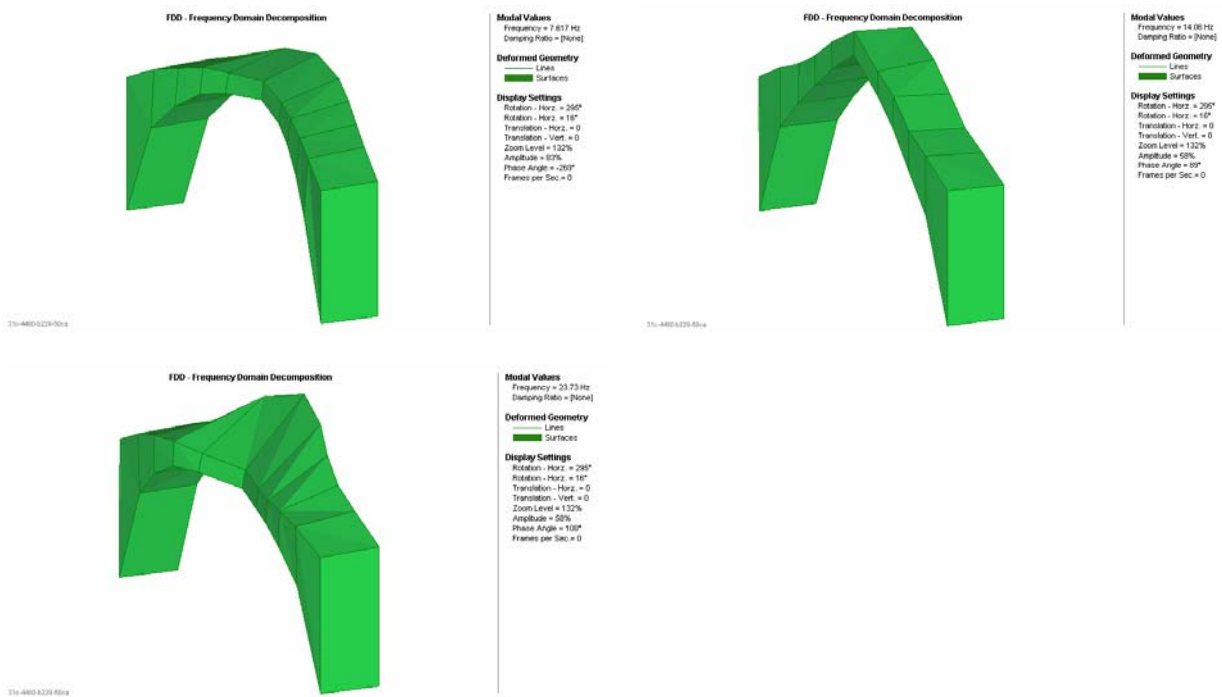
Figure 9 Shapes of vibration at dominant frequencies, transversal & vertical direction
