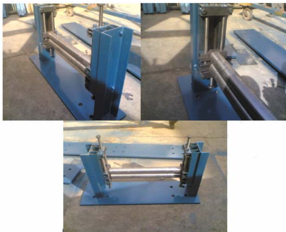
Figure 11. The rolling supports used at the beginning for preventing the frames from out-of-plane buckling
