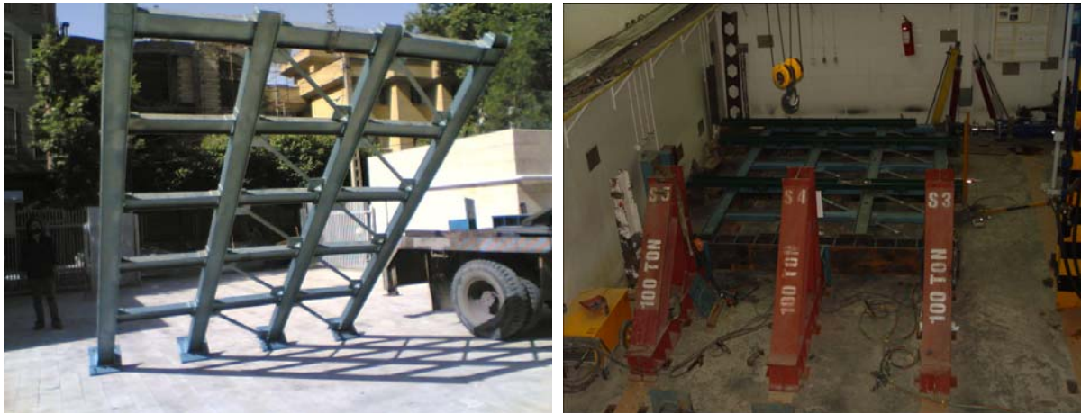
Figure 10. A framed of type III during shipment to the lab by lifer (left), and ready for test (right)
