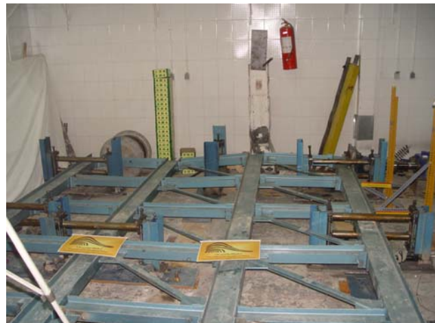
Figure 12. Buckling of a frame of type III in its second mode because of insufficient prevention
