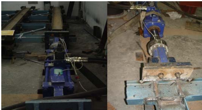
Figure 9. The used actuator in the tests and details of its support and connection to samples
