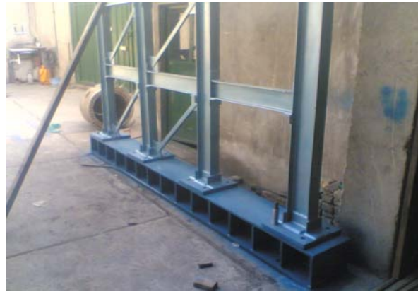
Figure 6. The relatively rigid beam used at the bottom of frames to act as their foundation
