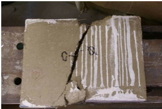
Figure 6: Unreinforced earth plaster panel specimen, after failure.
