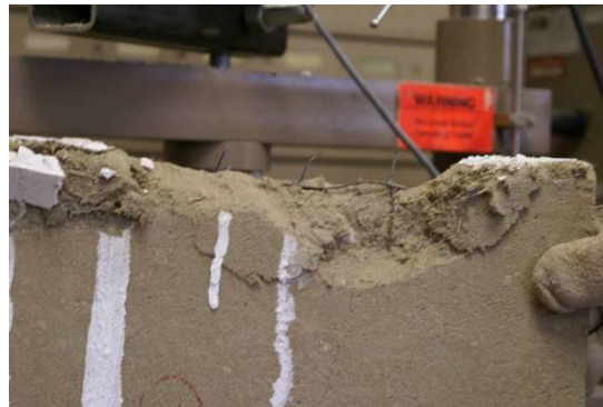
Figure 8: Reinforced shear panel specimen with showing edge failure under reversed cyclic loading
