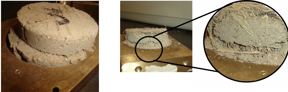
Figure 4: (a) direct shear specimen with defined shear plane; (b) close-up of embedded straw
