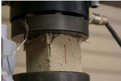
Figure 3: (a) cube compression test, and (b) Cintoflex C strand tensile test, showing failure and strand junction.
