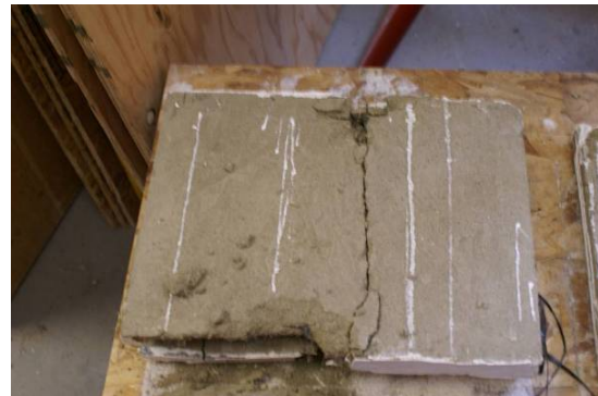
Figure 7: Earth plaster panel specimen reinforced with Cintoflex C mesh, after failure.
