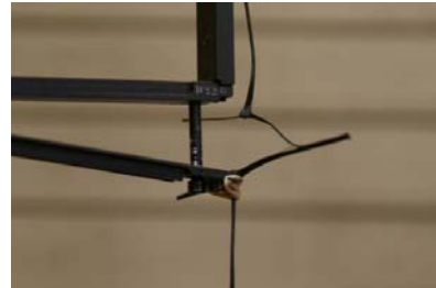
Figure 3: (a) cube compression test, and (b) Cintoflex C strand tensile test, showing failure and strand junction.
