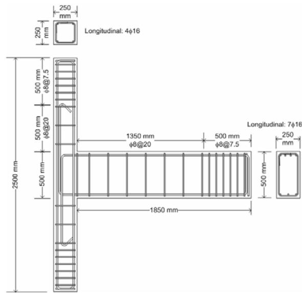
Figure 2.1 Reinforcement details for the test specimen
