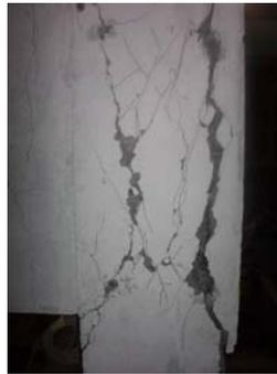
Figure 4.1 The cracks occurred in the joint region at the end of the test
