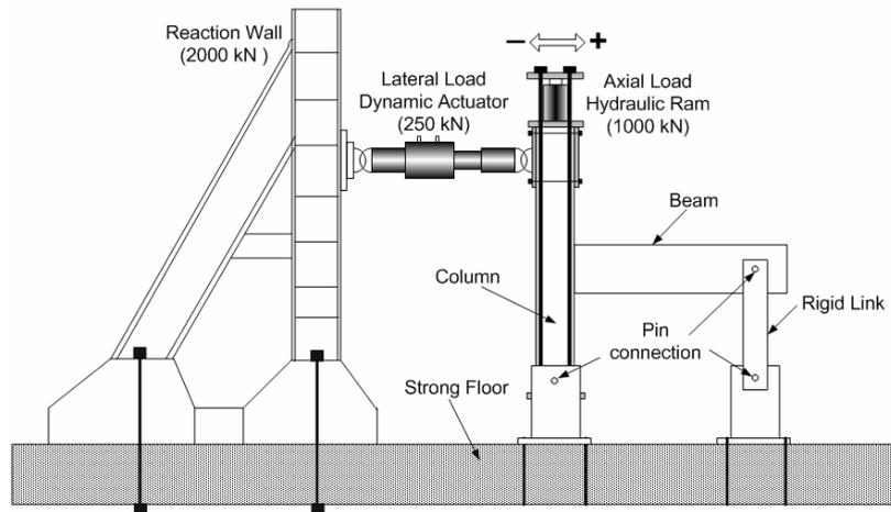
Figure 2.3 The test setup
