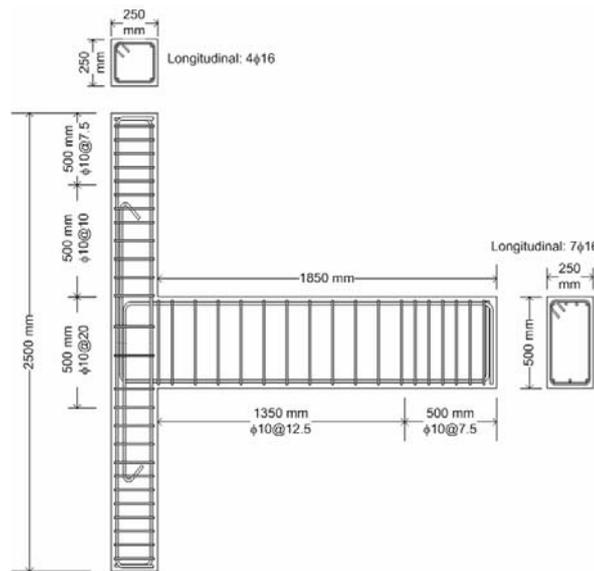
Figure 2.2 Reinforcement details according to TDY-75 code
