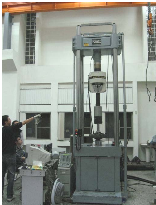
Figure 7 MR damper attached to a material test control system
