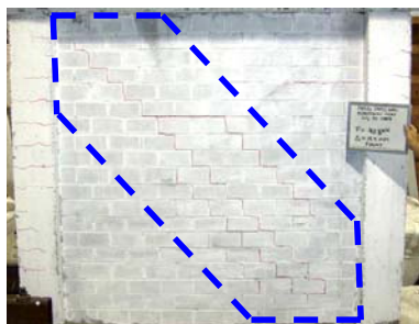
b) Diagonal Crack Pattern at 15 mm
