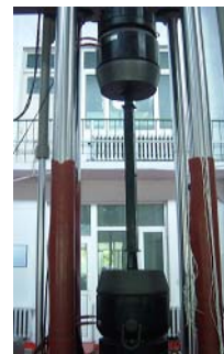
Figure 4. Photograph of experimental setup with BRB specimen
