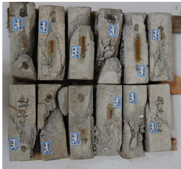
Figure 7: Failure type of specimens under dynamic loading
