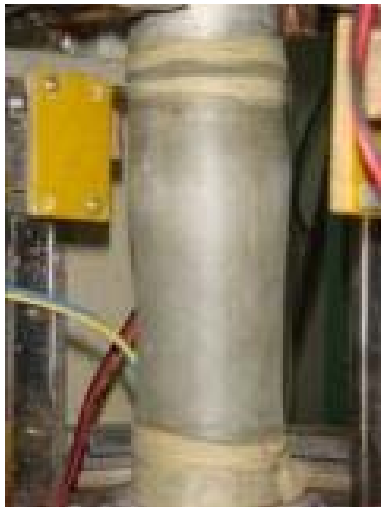
Fig.1 The swelling phenomenon of the sample
