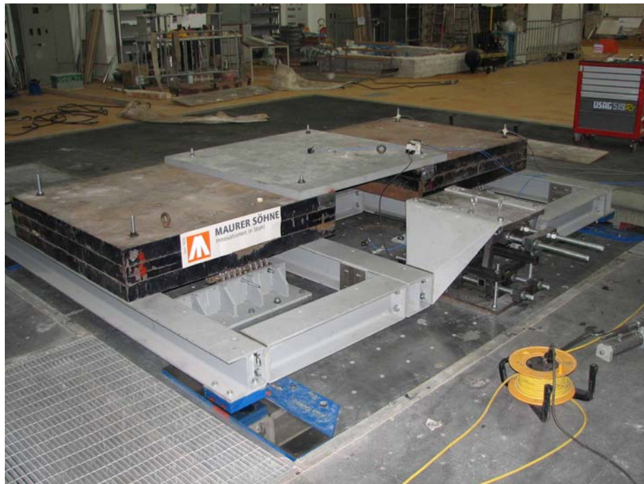
Figure 4: Testing rig for flat PTFE sliding bearings equipped with steel hysteretic elements. Reaction mass equal to 12,2 t
