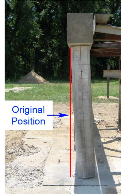
Figure 6 Column SJ2 after test
