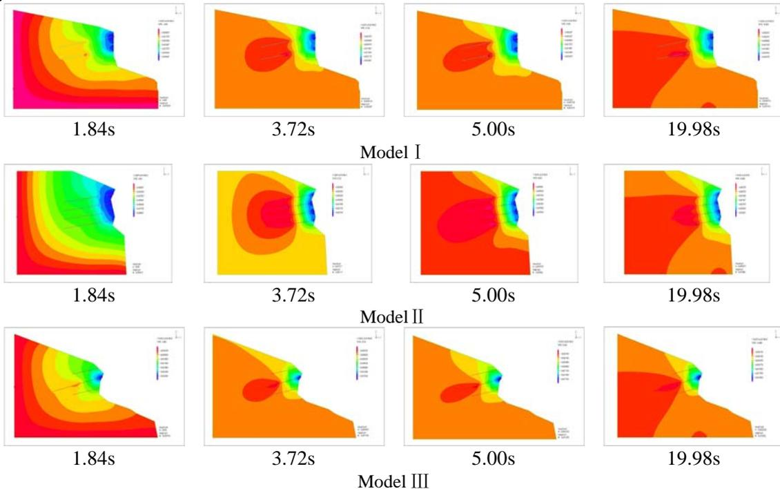
Fig.5 Displacement isograms in different moment for model I ,model II and model III ( $PGA=0.1g$ ,  $T_g=0.25s$ ,  $t=20s$ )
