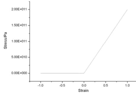
Fig.3 The graph of the stress and strain relationship of prestress anchor cable
