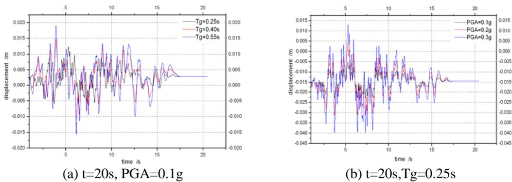
Fig.4 Time history of the displacement of the reinforced slope under different PGA or  $T_g$
