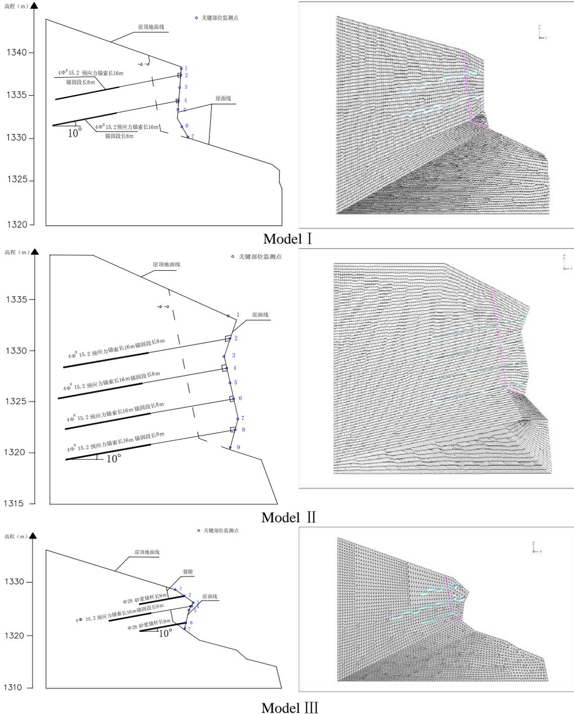
Fig.2 Design details and the finite element models
