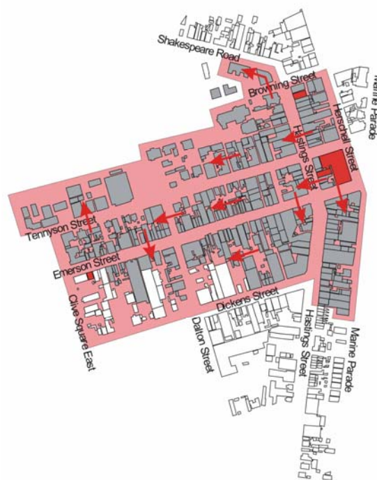
Figure 6 Plan of Napier CBD showing the path of fire spread in the simulation
