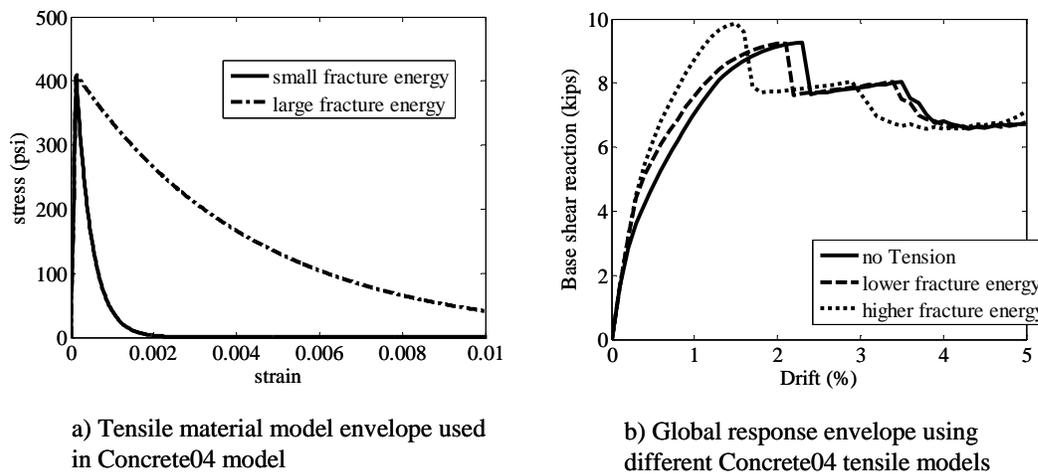
Figure 5. Effect of tension in pushover analysis of RC columns
