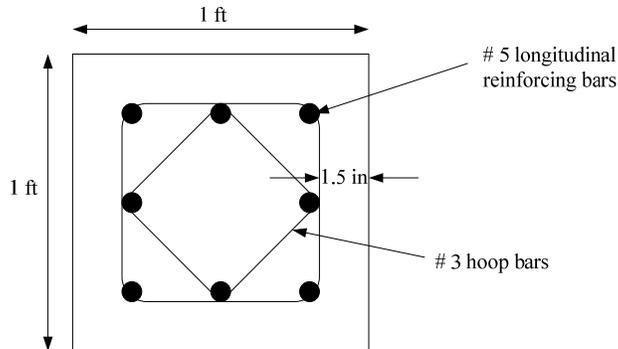
Figure 1. Reinforced concrete column cross section
