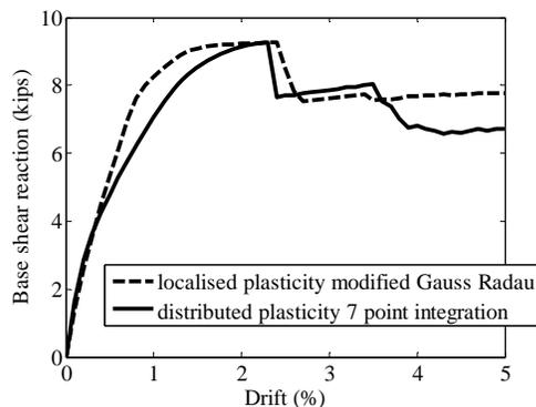
Figure 3. Comparison between RC column pushover response for lumped and distributed plasticity element formulation
