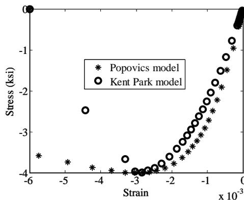
a) Concrete compressive envelope response with concrete empirical models
