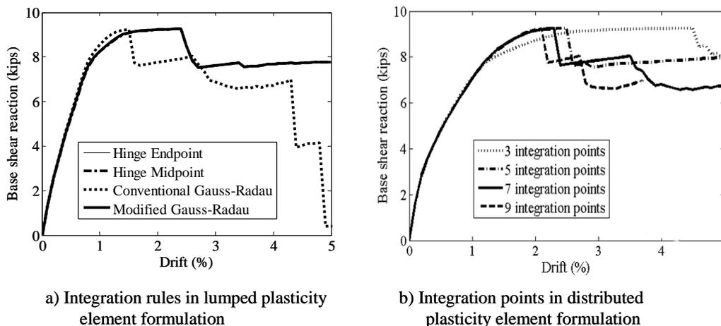
Figure 2. Variation in pushover response with integration rules along element length
