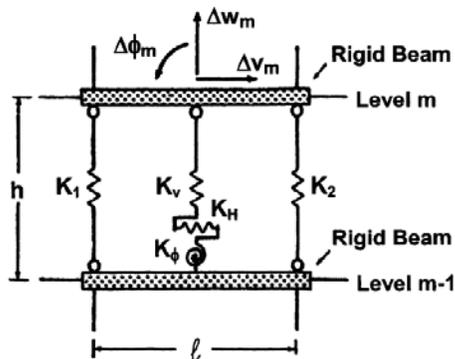
Figure 9 Three Vertical Line Element model (Kabeyasawa et al. 1983)
