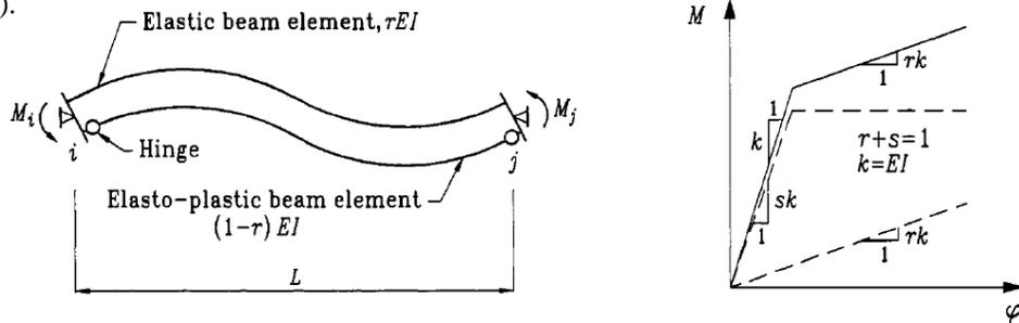
Figure 2 Two-component element model.
