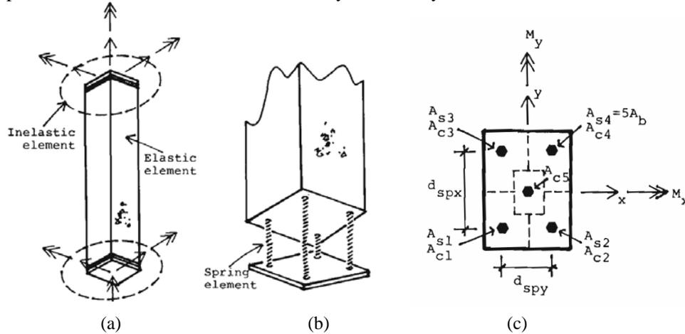
Figure 7 Multi-axial spring model by Lai et al. (1984): a) Member model, b) Inelastic element, c) Effective concrete and steel springs.
