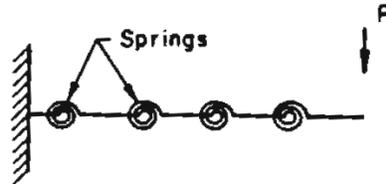
Figure 6 Multiple spring model (proposed by Takayanagi and Schnobrich 1976).
