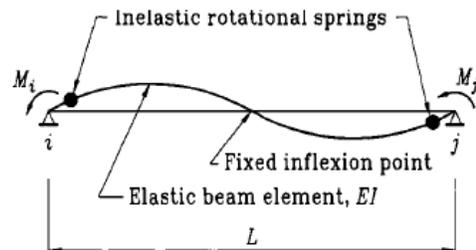
Figure 3 One-component element model.
