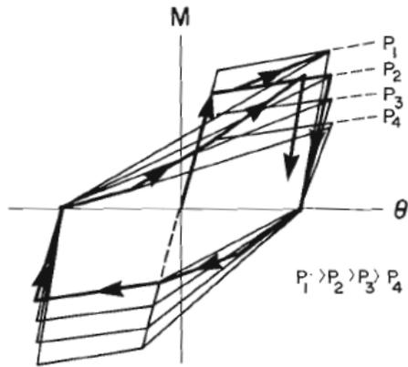
Figure 4 Hysteresis loops with effects of changing axial force (Saatcioglu and Derecho 1980).
