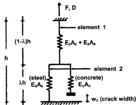
Figure 10 Axial-element-in-series model (Vulcano and Bertero 1986).
