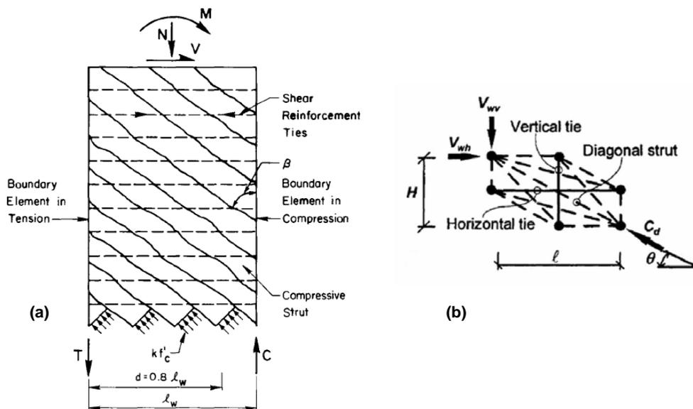
Figure 8 (a) Truss model used by Oesterle et al. (1984), (b) Softened-Strut-and-Tie model (Yu and Hwang 2005).
