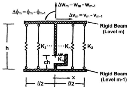
Figure 11 Multiple vertical line element model (Vulcano et al. 1988).
