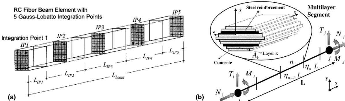
Figure 1 (a) Fibre beam element proposed by Monti and Spacone (2000), (b) Multi-layer finite element model (Belmouden and Lestuzzui 2007)
