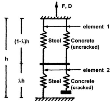
Figure 12 Modified axial-element-in-series model (Vulcano et al. 1988).
