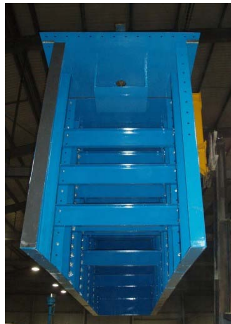
Figure 5: End view into Tsunami Generator tank before installation into the test facility
