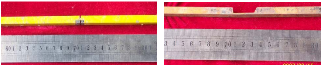
Photo 1 damage profile of member A (left) and member B (right)
