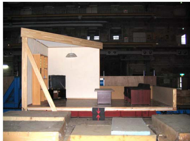
Figure 4 Set up of wooden table with furniture
