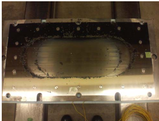
Photo 2 Surface of PTFE-Coated Stainless Plate after Testing (PTFE-Coat was peeled by friction)
