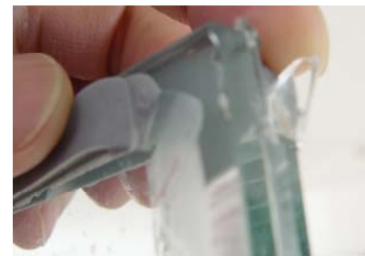
(c) Defect at glass corner
