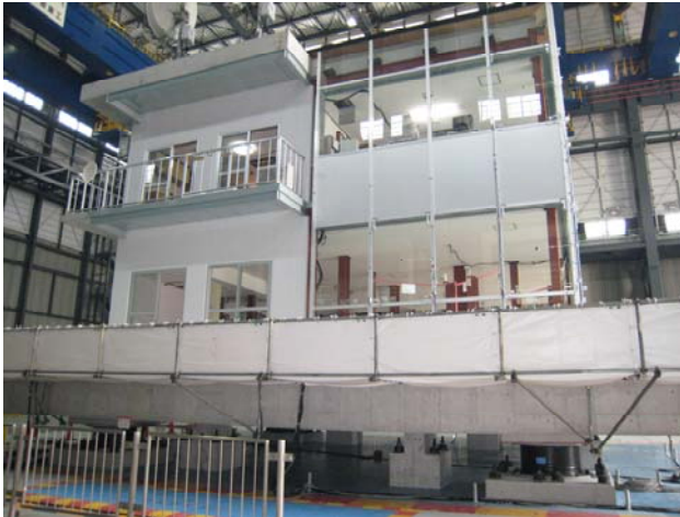
Photo 1 Test specimen for shaking table test
