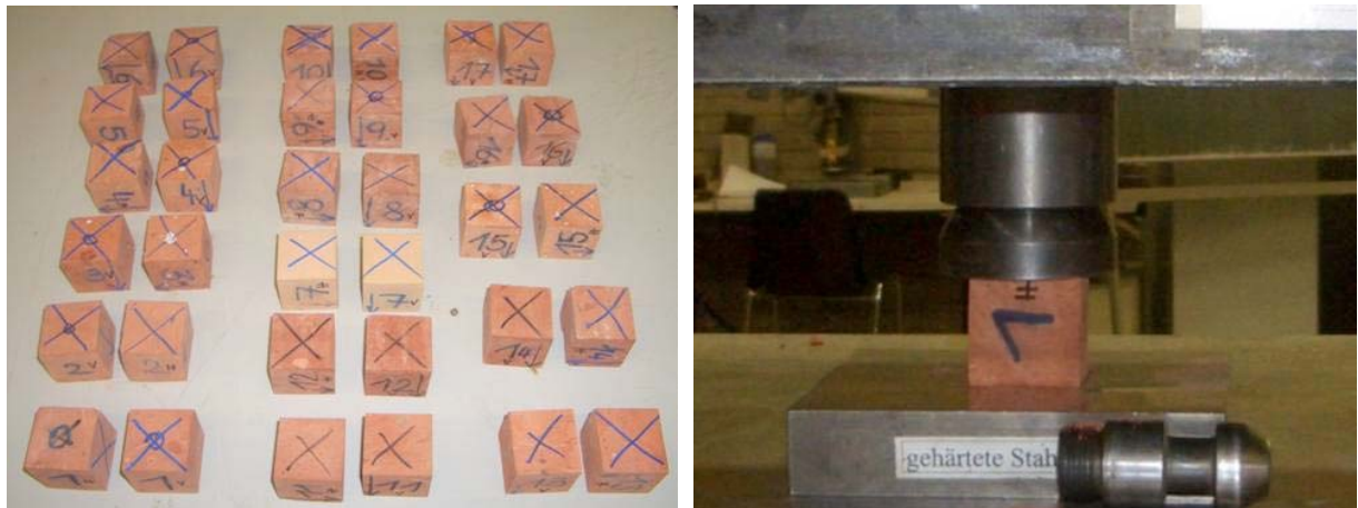
Figure 5 Laboratory testing of brick specimens in laboratory of the University of Innsbruck
