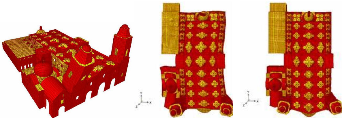
Figure 7 Vibration modes: (a) 16 th mode T=0.6s (b) 31 st mode T=0.45s (c) 34 th mode T=0.36s
