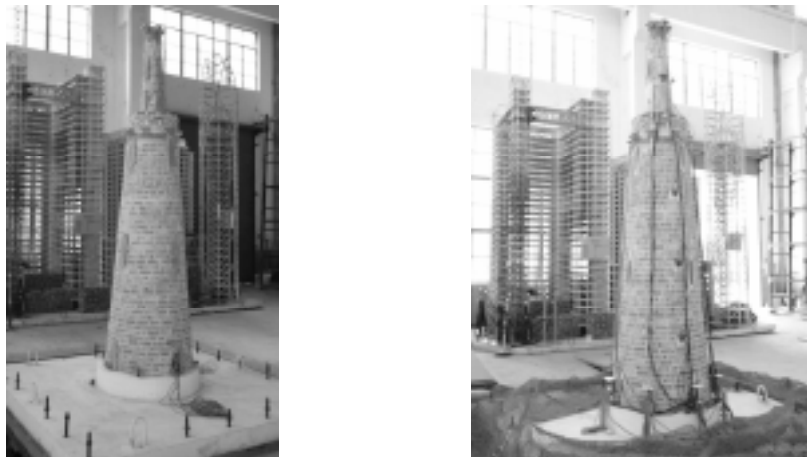
Fig.9 pictures of model structure with and without SMA dampers
