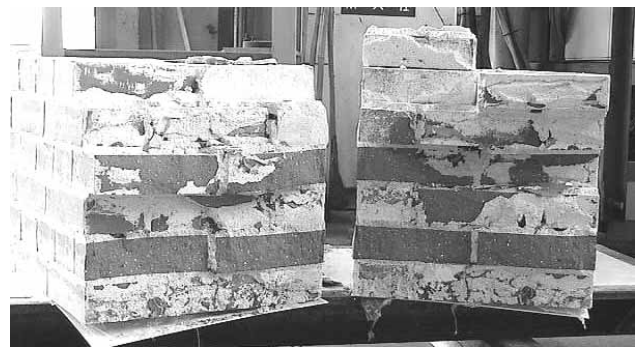
Figure 11: Failure appearances of test pieces
