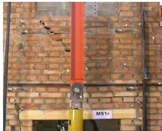
Figure 10. Specimen MS1r: (a) shear load against displacement, (b) crack pattern in the spandrel.
