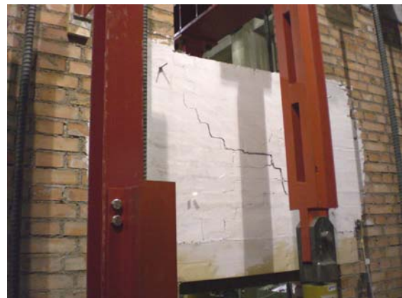
Figure 8. Specimen MS2: (a) shear load against displacement, (b) crack pattern in the spandrel.
