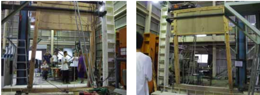
Figure 11 Full-scale wall test of wooden frame with hanging wall (No.1)
