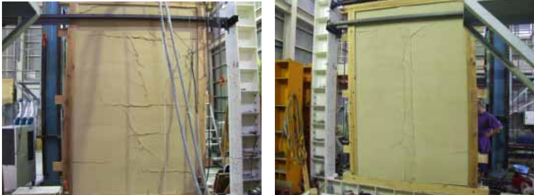
Figure 13 Full-scale wall test of mud plaster wall with 1820 mm length
