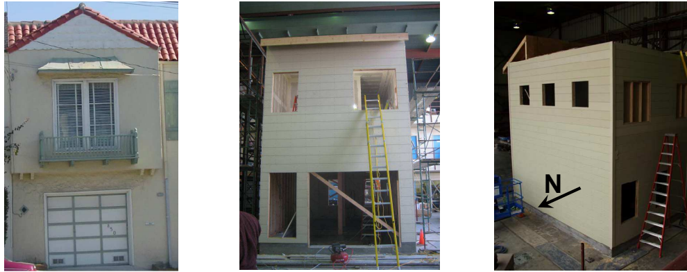
a) House in San Francisco b) Test building – east c) Test building – northwest Figure 1 Similarity between a typical San Francisco house and the test building
