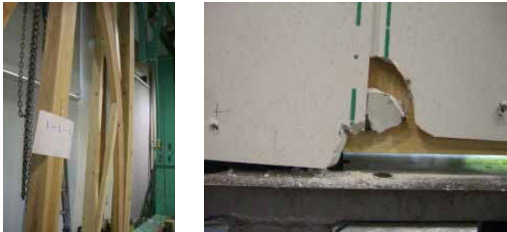
Photo 1 Failure mode (Left: Single brace, Right: MOISS)
